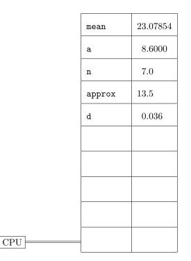
Data items are fetched one by one from the memory, are sent to the central processing unit (CPU) in which the actual computation is performed, and then the results are returned one by one to their 'cells'. The basic philosophy of the von Neumann machine is that data is 'normally' at rest.
